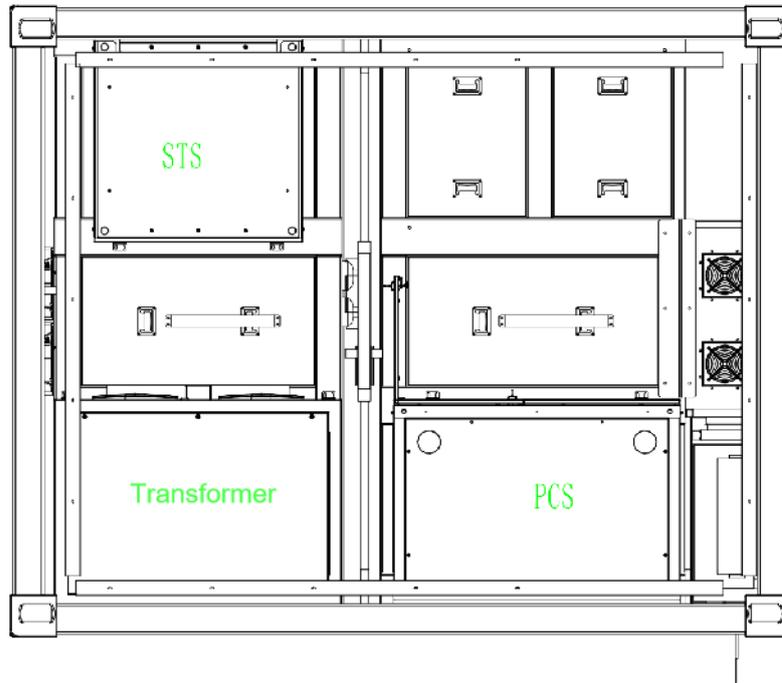
**Figure 3 Layout Diagram of AC Coupling Scheme**
