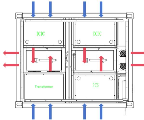
**Figure 14 Schematic Diagram of Forced Air Cooling System**
