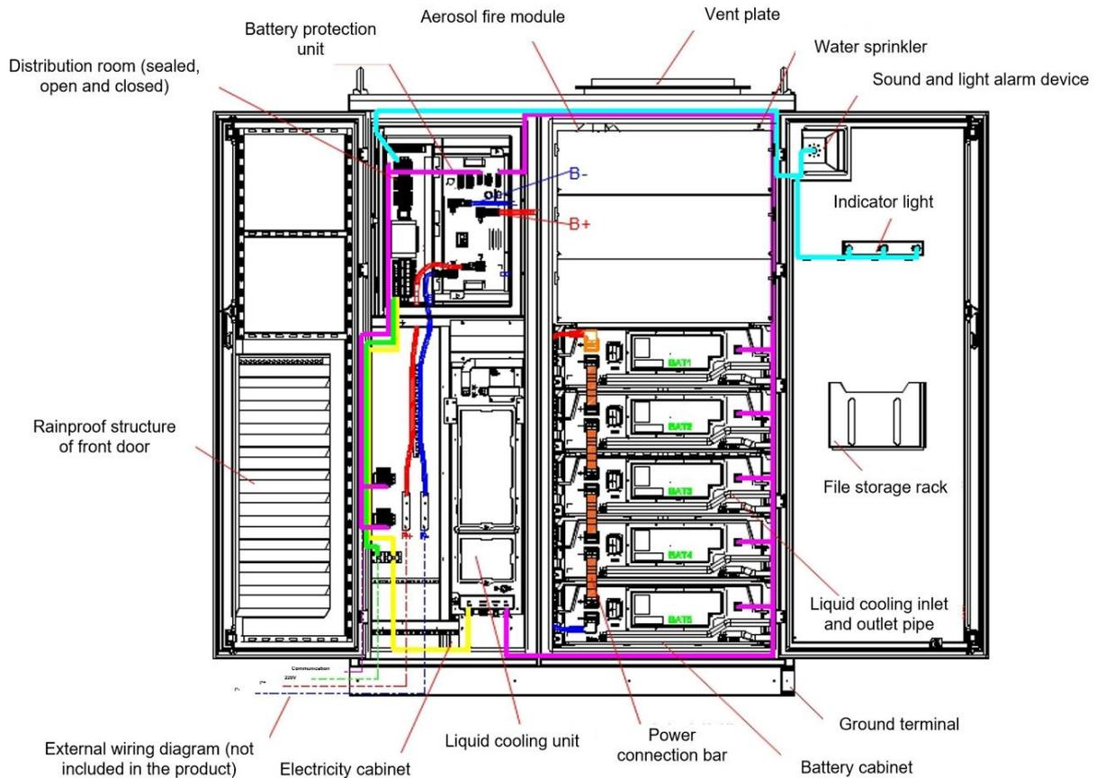
**Figure 1 Interior Layout Diagram of the Outdoor Cabinet**
