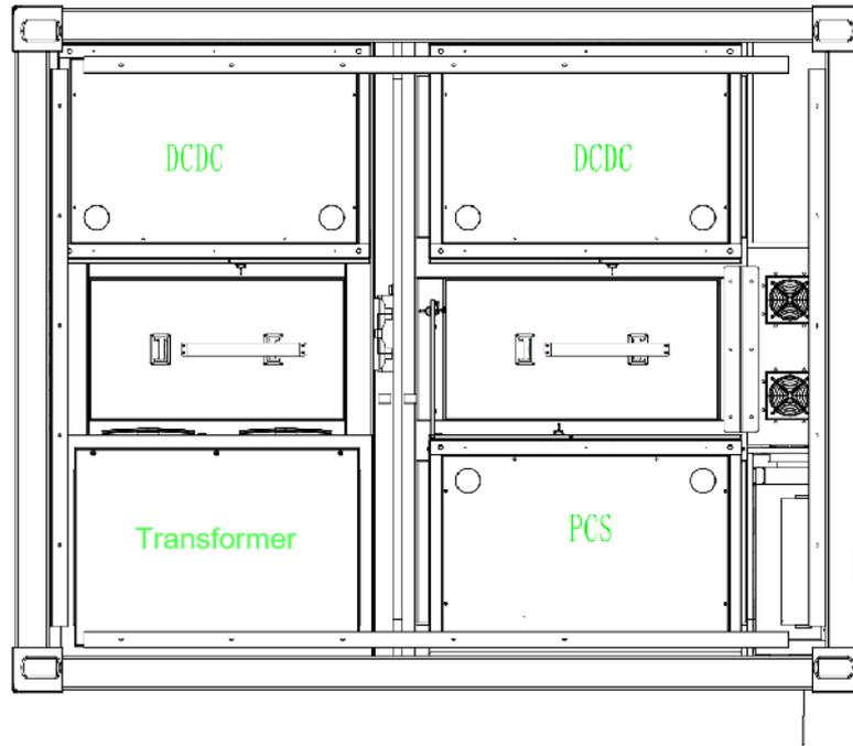
**Figure 2 Layout Diagram of DC Coupling Scheme**
