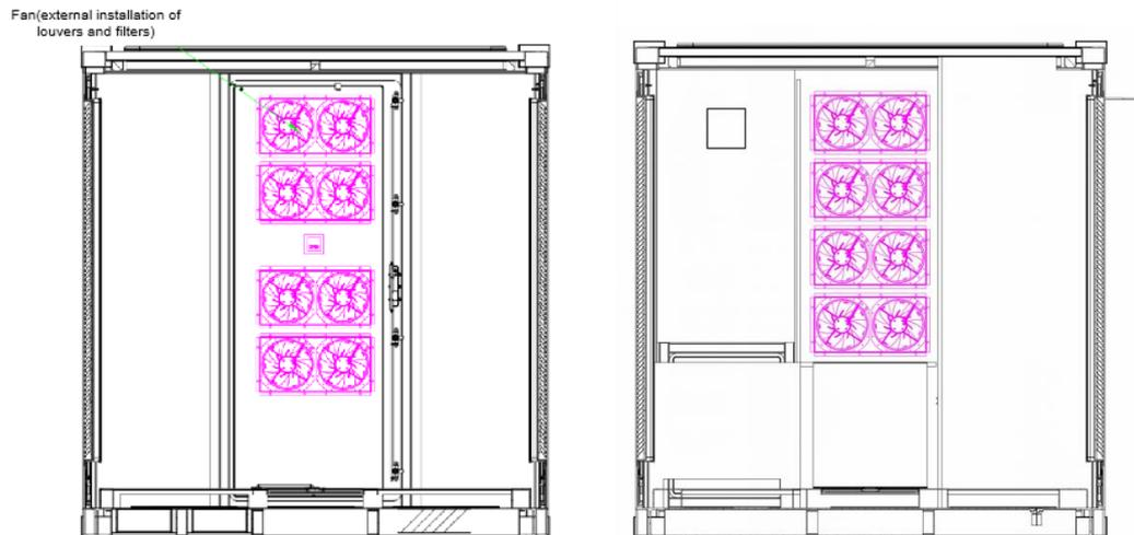
**Figure 15 Schematic Diagram of Fans**
