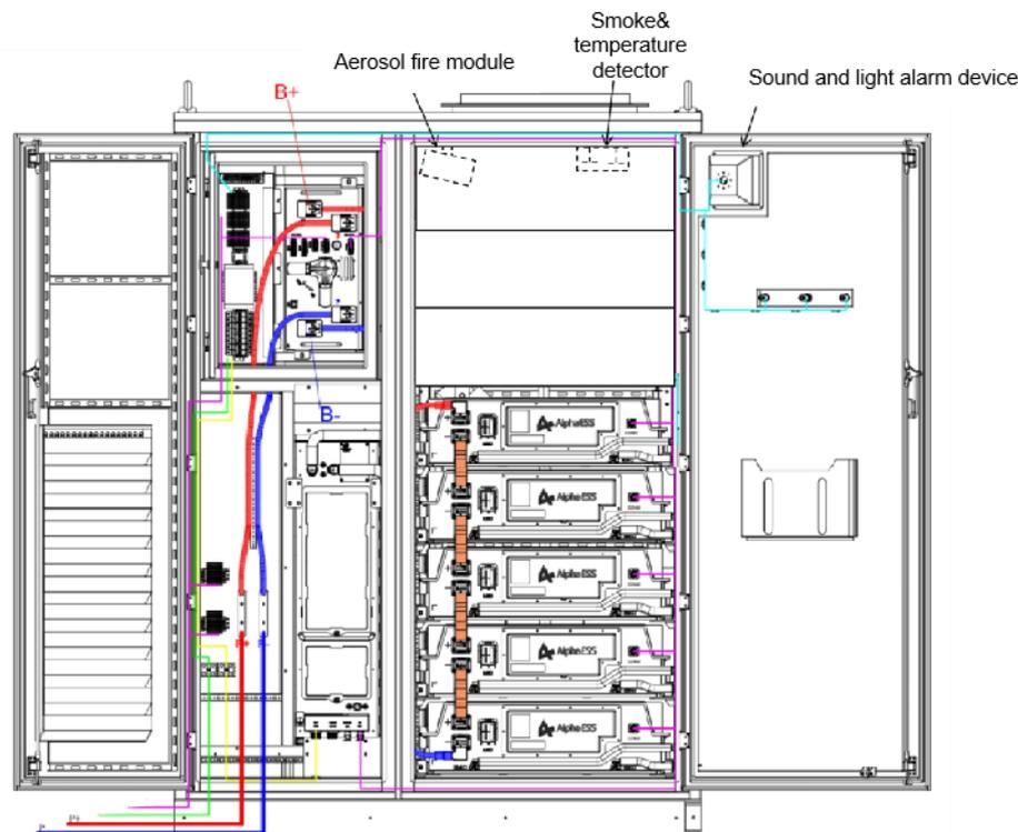
**Figure 16 Layout of Battery Cabinet Fire Protection System**
