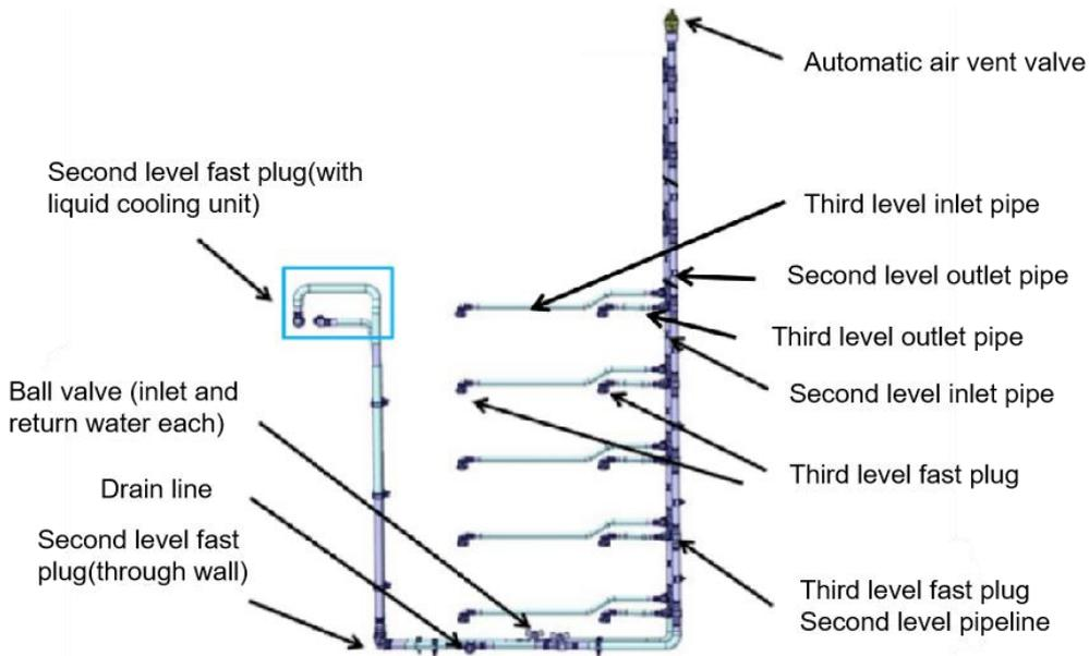
**Figure 13 Schematic Diagram of Liquid Cooling System**
